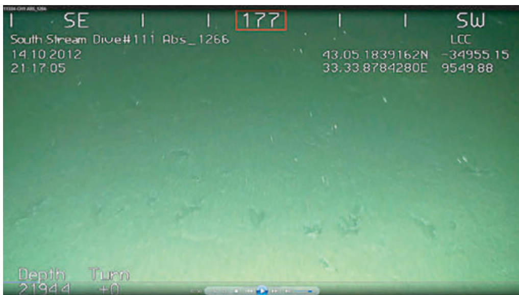
Figure 78. Still images derived from ROV video showing linear trails of furrows, pits and grooves cut into the modern soft seafloor flocc layer by objects carried across the seafloor by bottom currents.
