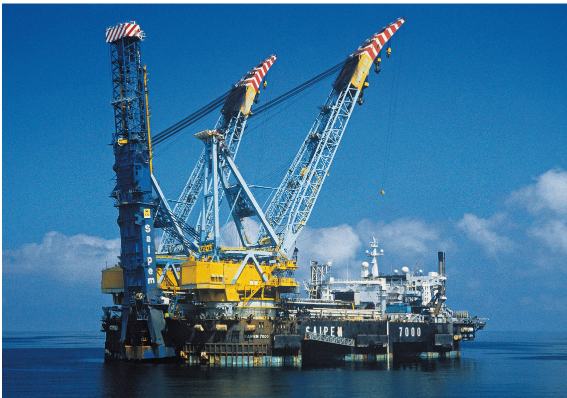
Figure 5.33 Typical Deep Water J-Lay Vessel
