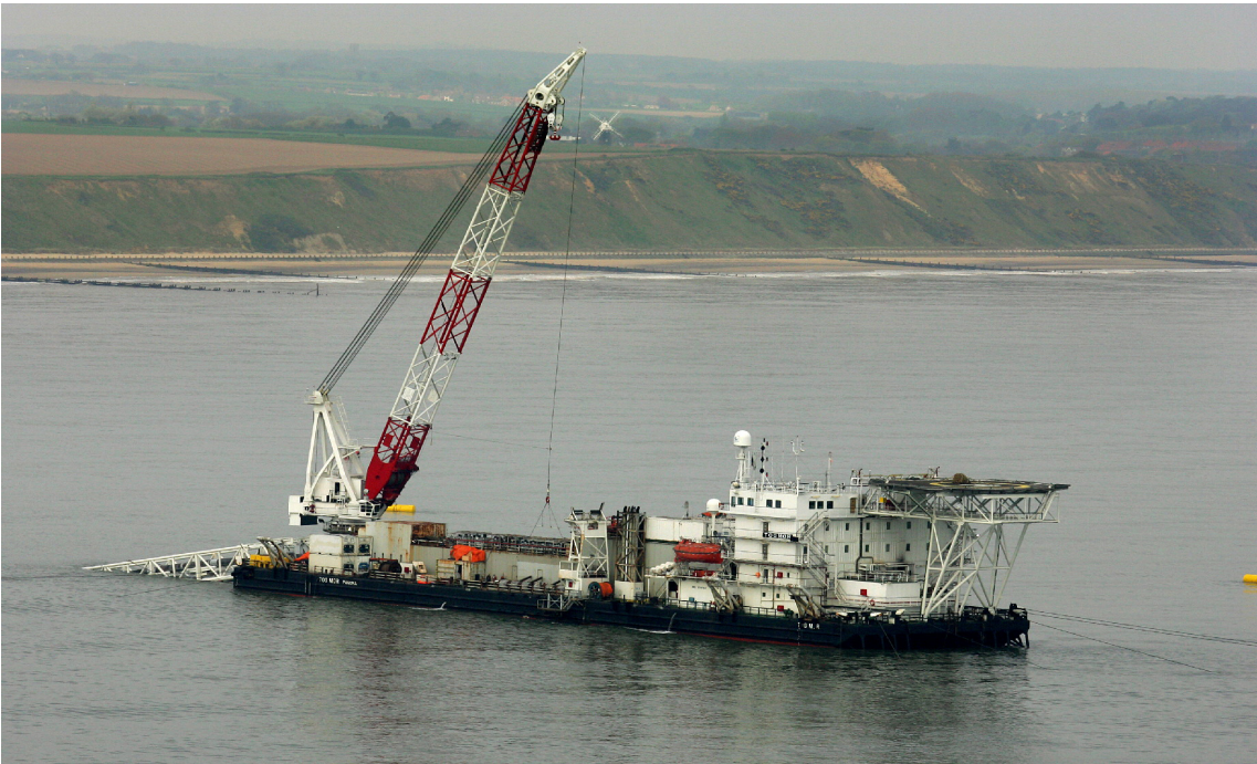
Figure 5.29 Typical Shallow Water S-Lay Vessel
