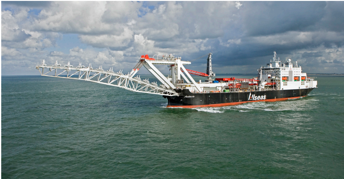
Figure 5.32 Typical Intermediate Water Depth S-Lay Vessel
